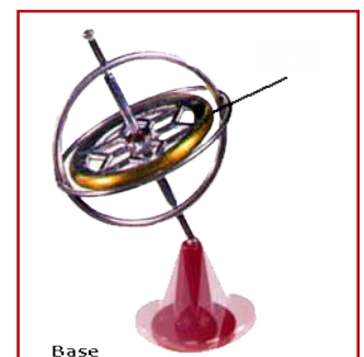
The spinning gyro will hold its position interdependent of the base motion.
